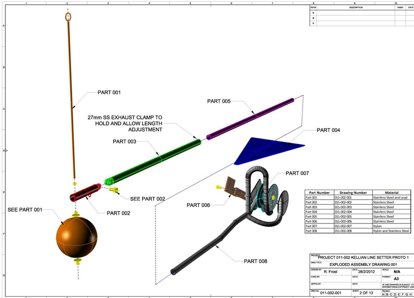
To provide a complete record of the initial prototype, we developed 'as built' drawings. The unit was measured, and 2D and 3D drawings of the initial unit produced. The primary dimensions allow for calculations of required weights/forces on key components, particularly the lead weight and paravane.
