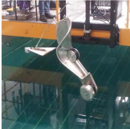
The initial KLS P2 attachment method tested was identical to the Prototype One configuration. Unfortunately it was found that the added hydrodynamic forces generated by the large cowling and funnel arrangement of the P2 could not be reasonably controlled by the paravane system used in P1 (Figure 4). Modifications were made as seen in Figure 5 to increase the unit's towed stability.
