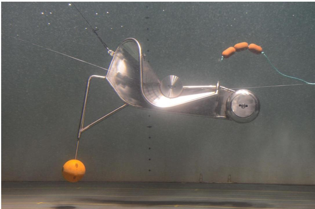
**Figure 4.** Kellian Line Setter P2 with paravane system attached.
